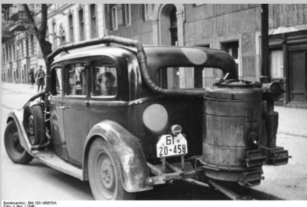
Car running on wood gas, Germany, 1944
